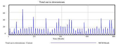
Fig. 8. Input discharge entering the Urmia Lake after lavian Dam construction.
