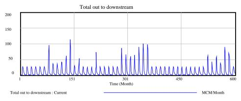
Fig. 18. Input discharge entering the Urmia Lake after Shahrchay Dam construction.
