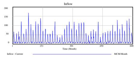
Fig. 17. Input discharge entering the Urmia Lake before Shahrchay Dam construction.
