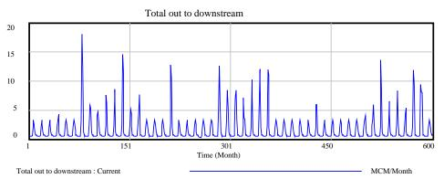
Fig. 10. Input discharge entering the Urmia Lake after Nahand Dam construction.
