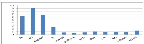
Fig. 2. Average monthly discharge of the river at the entrance to Nahand Dam (mcm).
