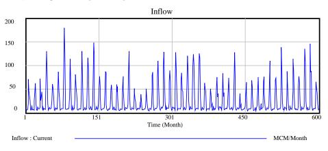
Fig. 15. Input discharge entering the Urmia Lake before Mahabad Dam construction.
